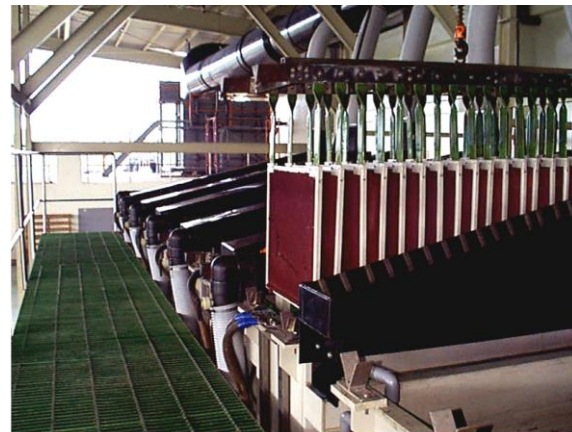
The full scale electrolytic copper recovery system (華通電腦) 陰極面積=60m 2 ；操作電流=12000A
